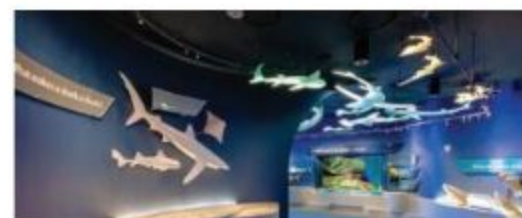
In the informative "Meet the Shark" area acrylic shark pendants are edge-lit with cool white Luminii LED tapelight to create a playful environment.
